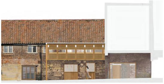
$Rendered\ sectional\ elevation\ cut\ through\ proposed\ foyer\ Link\ looking\ towards\ the\ North\ Range$
