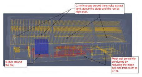
Figure 54: Mesh cell sensitivity study around the auditorium on the lower level
